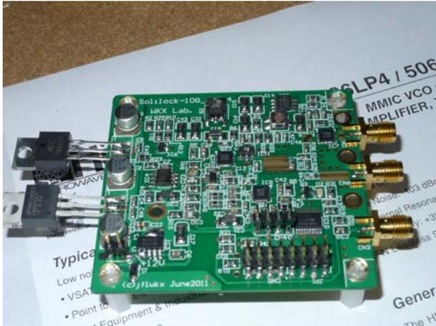
Photo 1 Entire circuit placed on a board, including RF circuitry (oscillator, multiplier, and PLL), controller, power supply, and PLL loop filter
